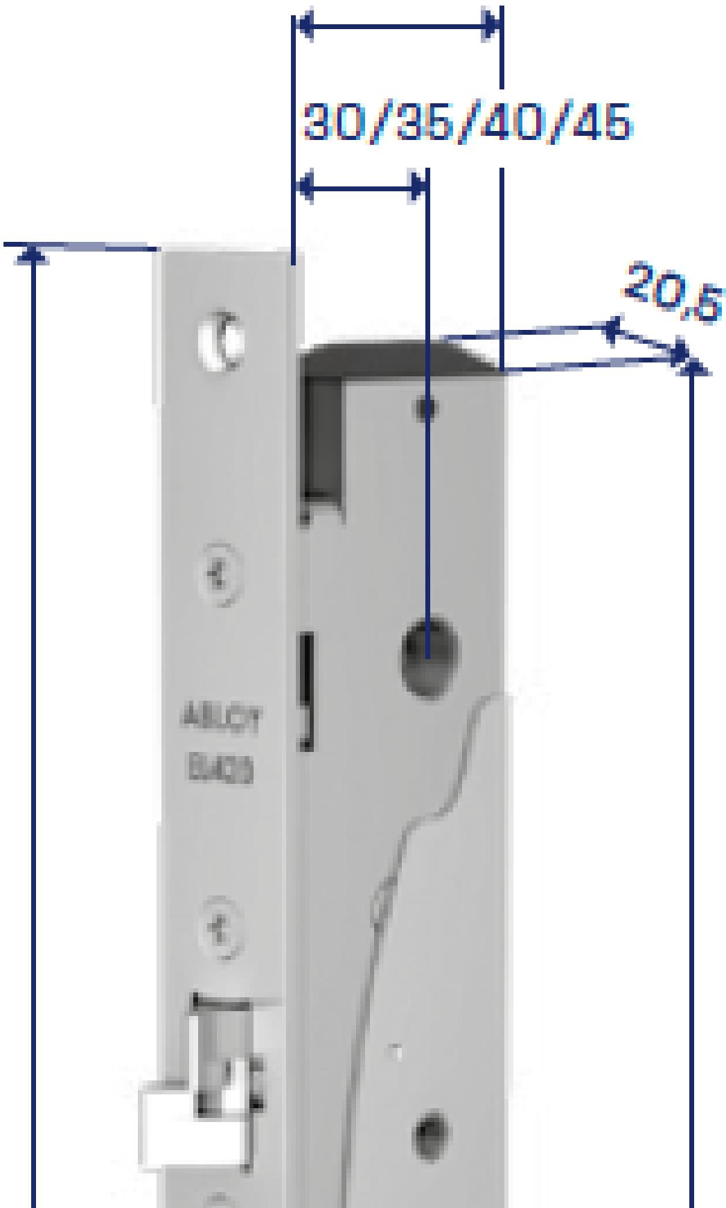
Diagram illustrating the dimensions of the KEL420 lock body. The top horizontal dimension is 45/50/55/60. The middle vertical dimension is 30/35/40/45. The bottom horizontal dimension is 20,5.
